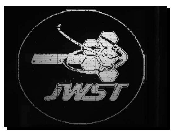
NIRSpec Microshutter array configured to specific pattern of open and closed shutters.
