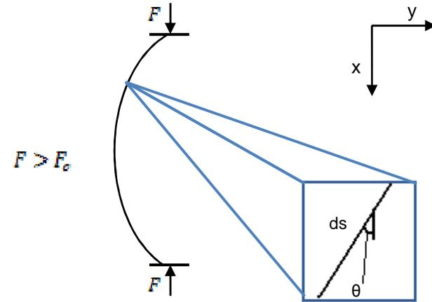
$$A \frac{d\theta}{ds} = -Fy \quad \Rightarrow \quad A \frac{d^2\theta}{ds^2} = -F \sin \theta \quad \Rightarrow \quad H = \int_0^L ds \left[ \frac{A}{2} \left( \frac{d\theta}{ds} \right)^2 + F \cos \theta \right]$$
