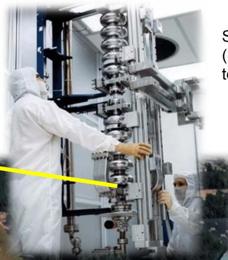
Superconducting radiofrequency (SRF) cavities undergo vertical testing.
