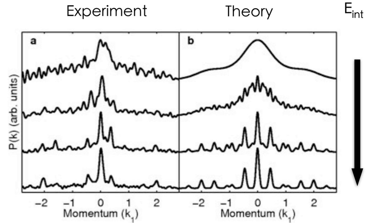
Adding interactions the momentum distribution becomes narrower: transition from a localized to extended state!
