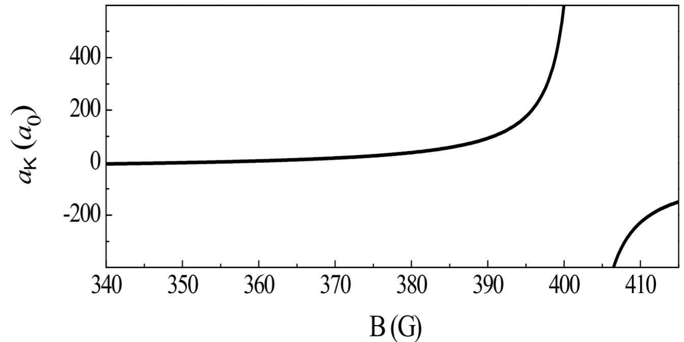
Tuning the interactions via a magnetic Feshbach resonance in a potassium condensate ( $^{39}\text{K}$ )
