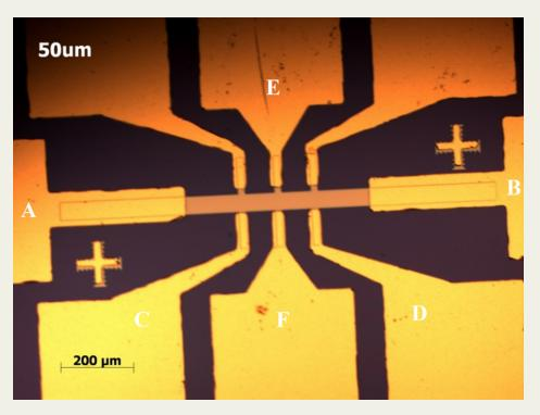
Current is injected through A and B
