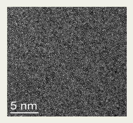
The HRTEM image of the amorphous  ${\rm Tb_{26}Fe_{64}Co_{10}}$  thin film by Titan 300 kV
