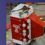
Threshold Čerenkov: Determined speed of particles passing through it via the Čerenkov effect, to differentiate electrons and positrons from much heavier pions.
