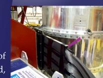
Front Tracker: Gave position of particles close to target magnetic field, to differentiate electrons and positrons.
