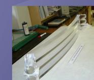
Lucite Hodoscope: Determined position of incoming particles and allowed background rejection.
