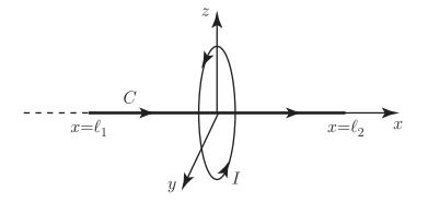
(a) The magnetic field along the x-axis due to the current loop of radius a in the yz plane is given by
