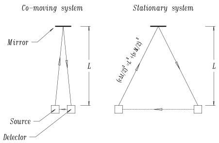
source emits a short pulse of light that bounces off the mirror into the detector. When the detector receives the pulse it immediately triggers the source to emit another one.
