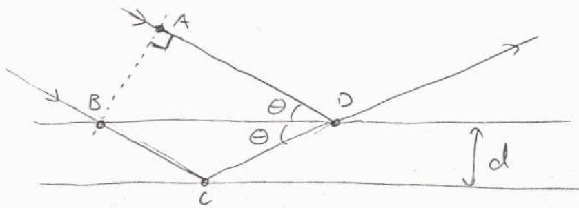
Dotted line shows input wave front = surface of constant phase
