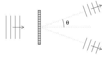
Implement with glass plate, sinusoidal markings simple diffraction grating
