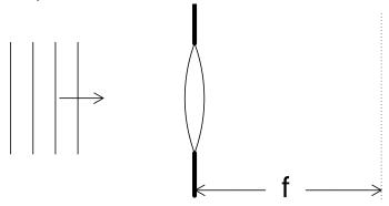
Plane wave incident on lens diameter D
