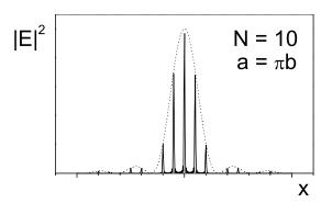
Sharp lines useful for spectroscopy
