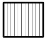
${f E}$  aligned with wires: drive current resistance ightarrow power dissipation ightarrow absorption
