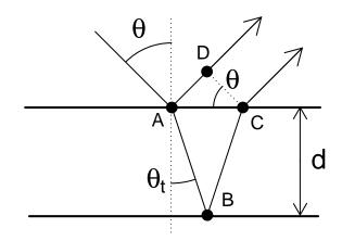
OPL for  $E_1 = \overline{AD}$ OPL for  $E_2 = n(\overline{AB} + \overline{BC})$
