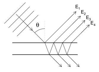
When R is not small, need to sum all reflections Mirrored plate = Fabry-Perot interferometer
