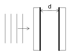
Scan mirror separation d: Large transmission when  $d = m\lambda/2$
