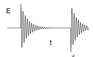
Typical atomic decay time = 10 nsMakes field that is *coherent* over 10 ns timescale
