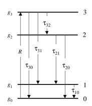
2. Gain Coefficient: Suppose that the system of problem 1 describes a solid state laser medium with the following data:
