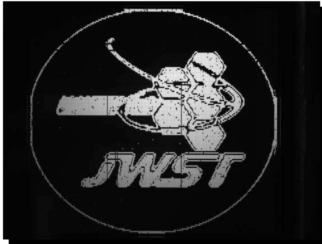
**NIRSpec Microshutter array configured to specific pattern of open and closed shutters .**
